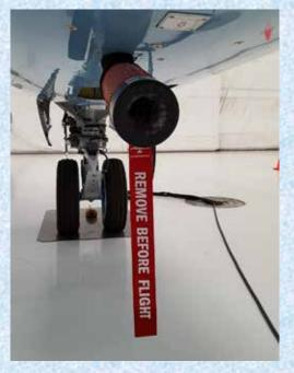
Check out and get one of our Boeing 737 Electrical/Electronics Exhaust Muffler for cooling compartment exhaust. Silence that loud EE exhaust while on the ramp. Reduce the loud E/E fans dumping overboard under your Boeing by up to 70% with our custom muffler. Fast and easy to install and remove. Also prevents birds nesting in there while parked on the ramp.
