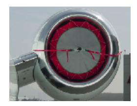
Venting Type - Dual: 1 mesh + 2 trampoline valve to relieve
